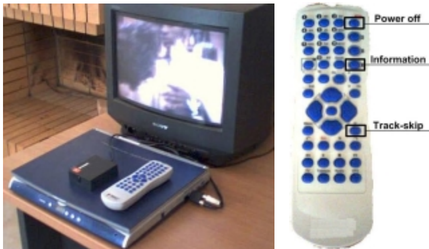
Figure 16 A low-budget set-up for interactive television usability evaluation consists of a portable computer, an infrared receiver, a normal remote control and an audiovisual cable to connect to the TV
