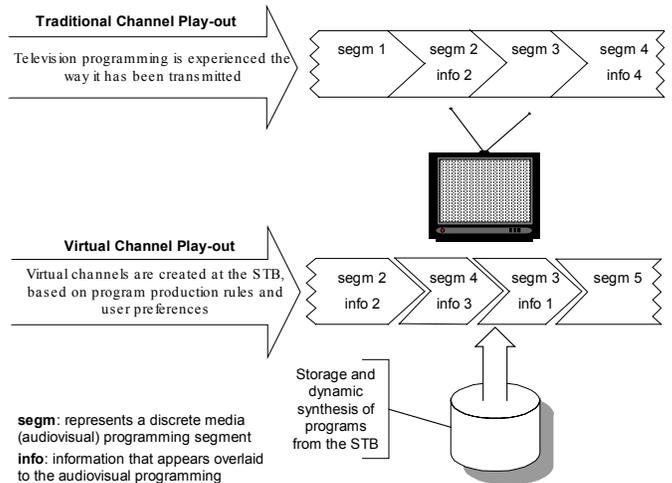
**Figure 1** Generic model of a system employing the virtual channel model, in contrast with traditional broadcasting
