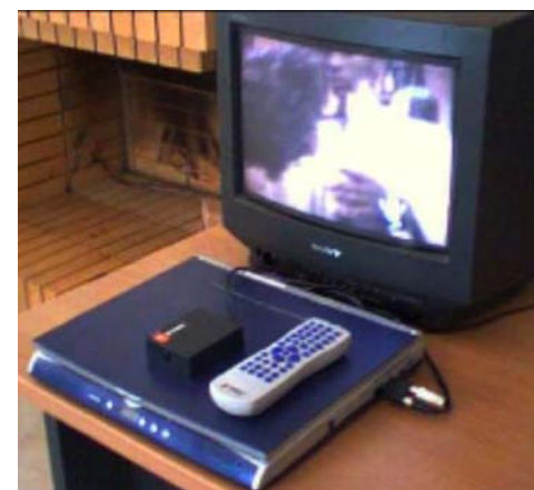
Figure 2 The experimental setup is seamless and unobtrusive, because it consists of conventional TV set, remote control. The portable computer, which controls the ITV prototype, could be easily hidden away
