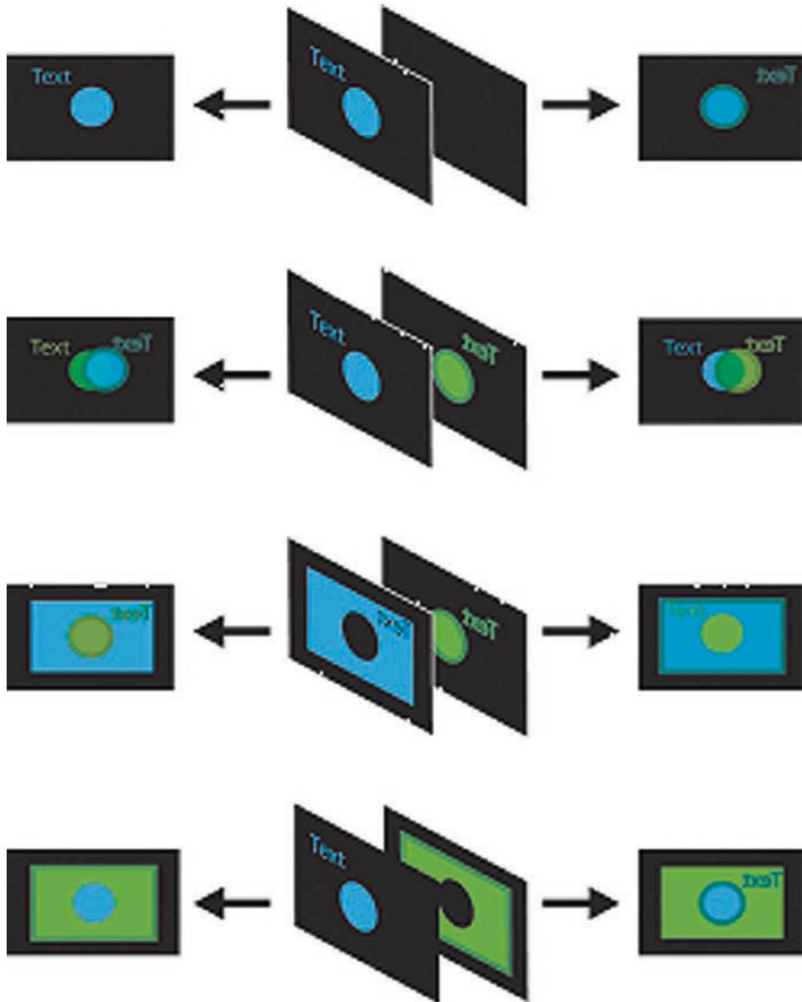
Fig. 5.3 Examples of different types of color mixing on a double projection system
