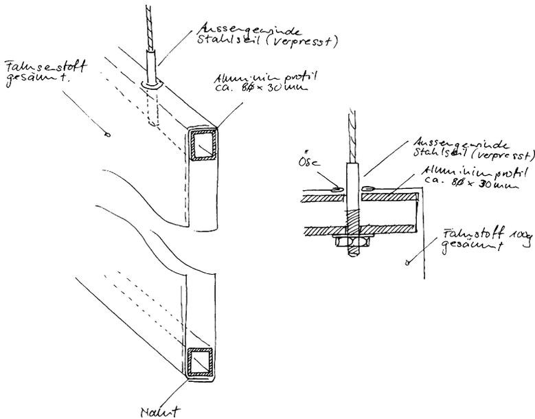
**Fig. 5.6** The double projection screen consists of two sides of semi-transparent white textile material arranged in parallel to each other and organized in the same frame, which is lightweight enough to hang from two metallic threads; thus it looks like it is hovering
