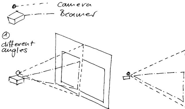
Fig. 5.8 Camera and projector are positioned together
